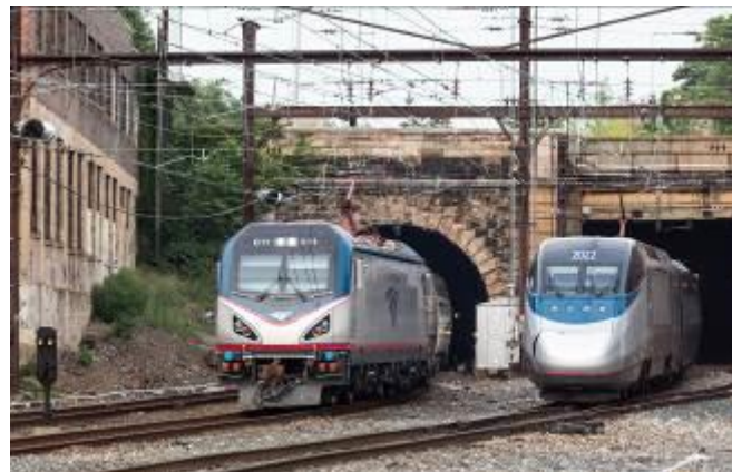
A train pulled by a new Amtrak Cities Sprinter (ACS-64) electric locomotive (l) and the Acela Express meet at Baltimore.
